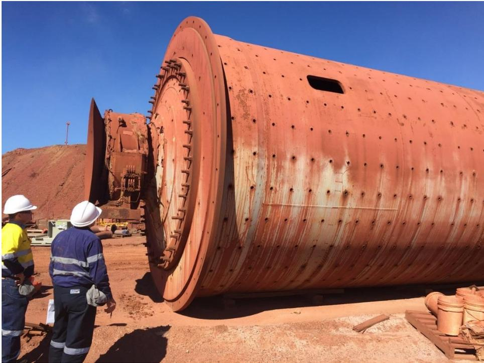
**Figure 1. The 2.5MW Ball Mill Shell 60km from LGP**
