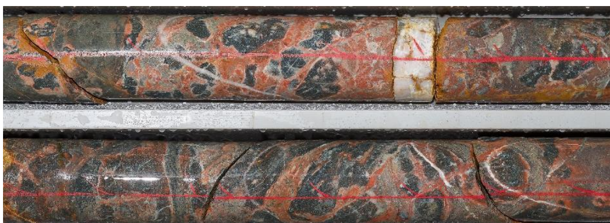
Figure 9. BL18DD018 from 57.4 metres. Broad zone of strong Potassium Feldspar (Orthoclase) alteration with quartz-carbonate veining and disseminated sulphide. Grading 1.4 g/t Au, 3.2 g/t Ag, 0.09% Cu.
