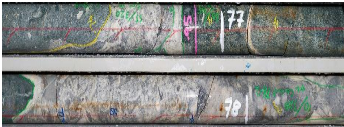
Figure 7. BL18DD017 from 76.5 metres. Low sulphidation epithermal boiling zone textures with internal metal veining.
