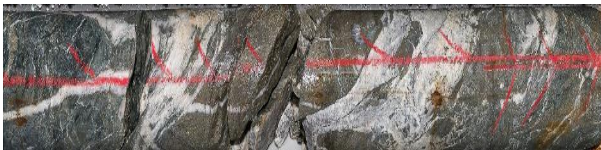
Figure 4. BL18DD018 from 96 metres. Gold rich massive sulphide grading 6.6 g/t Au, 36.5 g/t Ag, 0.2% Cu, 7.0 g/t Te and anomalous As, Bi, Pb, Sb and Zn.
