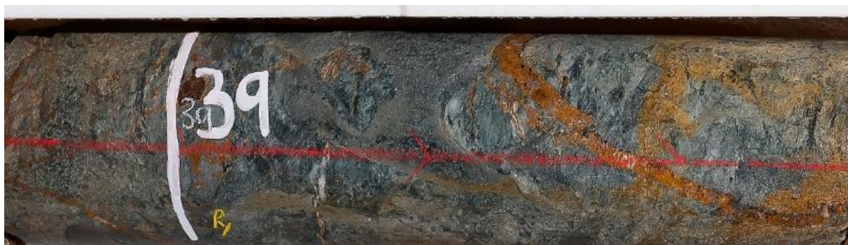
Figure 6. BL18DD014 from 38.8 metres. Altered sediment with fine sulphide grading 11.0 g/t Au, 6.1 g/t Ag with anomalous Mo, Sb and Zn.
