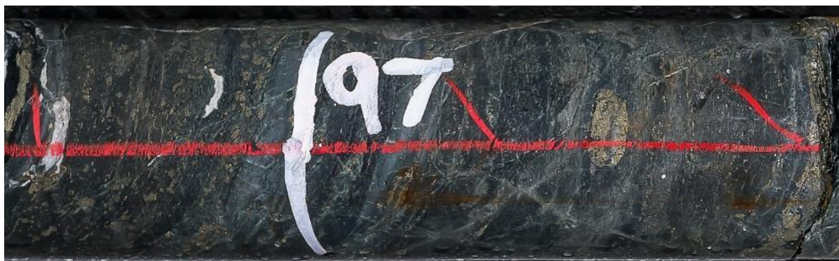
Figure 5. BL18DD018 from 97 metres. Siliceous sediment with banded sulphide and pyrite nodules. Grading 2.2 g/t Au, 3.2 g/t Ag, 0.2% Cu and anomalous As, Bi, Ni, Pb and W.
