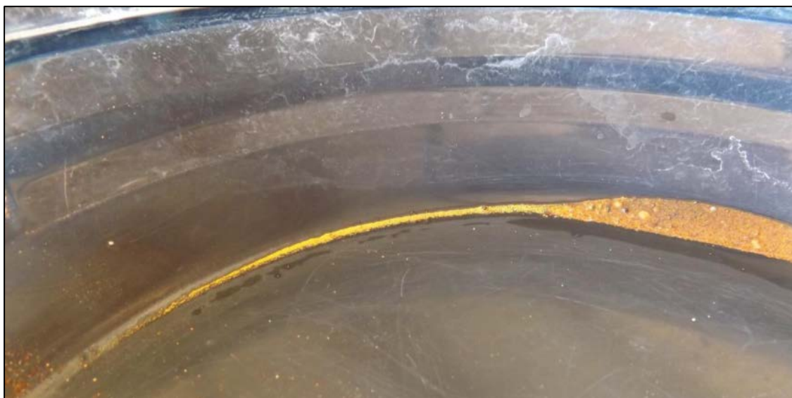
Figure 5: Gold tail in plan from East Lynne Prospect, from about 0.5kg of material
