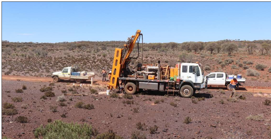
Figure 1: Aircore drilling currently underway at Cardinia Hill targets within the Cardinia Gold Project
