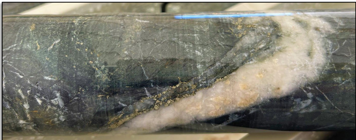
Figure 4: Mount Flora drill core showing silica-biotite altered basalt with quartz-carbonate veining containing scheelite (tan coloured mineral within the vein) and pyrite mineralisation at 188.6m hole depth. Photo is part of a 2.6m long zone grading 1.6% S, 580ppm W and 8.84g/t Au
