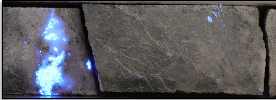
Figure 5: Mount Flora drill core under UV light showing scheelite (fluorescent blue colour) in silica-biotite altered basalt with quartz-carbonate-scheelite veining at 188.6m hole depth.
