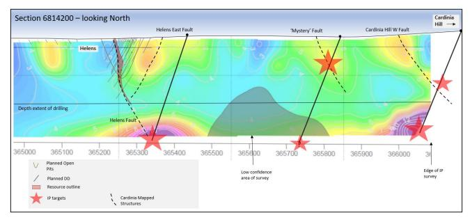
Figure 2 – IP cross section 6814200mN showing positions of proposed diamond drill holes
