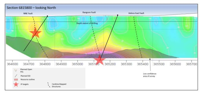
Figure 3 – IP cross section 6815800mN showing positions of proposed diamond drill holes
