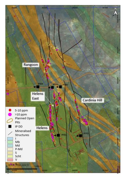
Figure 3 – Geological Plan of the Eastern Corridor deposits, highlighting the location of high-grade (+5.0g/t and +10.0g/t Au) drill intersections, structural interpretation and IP001 to IP005 diamond drill hole collar positions. Note the extent of high-grade intersections along the Helens-Rangoon Fault which extends for approximately 3.0km. Other adjacent faults (eg Helens East and Cardinia Hill Faults) also display extensive high-grade intersections where drilled.
