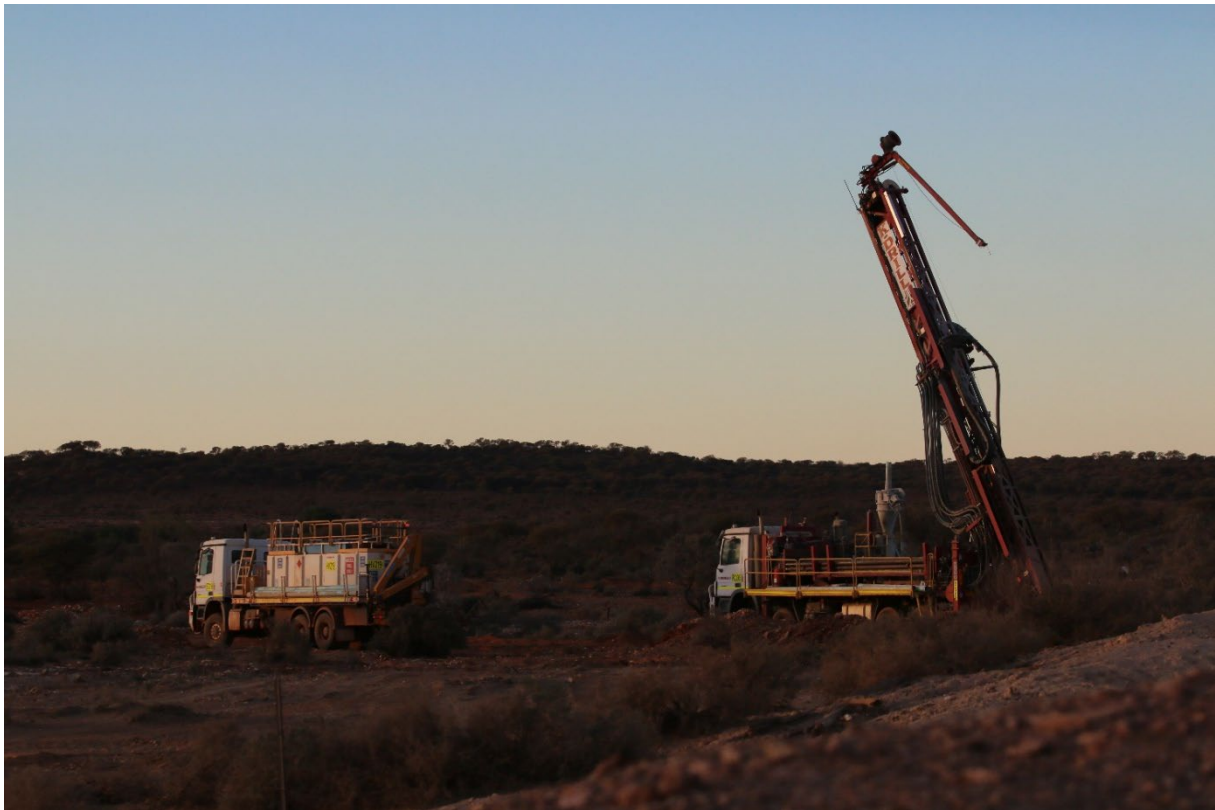
Figure 4 - K Drill RC rig currently drilling at East Cardinia.
