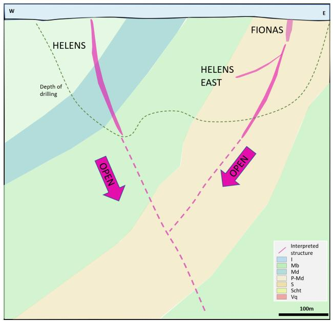
Figure 5 – Schematic cross-section looking north through the Helens – Helens East deposits, showing the interpreted interaction at depth. There is no drilling information below 200m.
