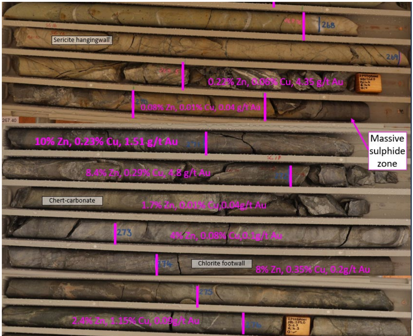
Figure 4 – IP22DD001 core showing sample intervals and latest results along with previous gold results (reported in ASX announcement 15 December 2022).
