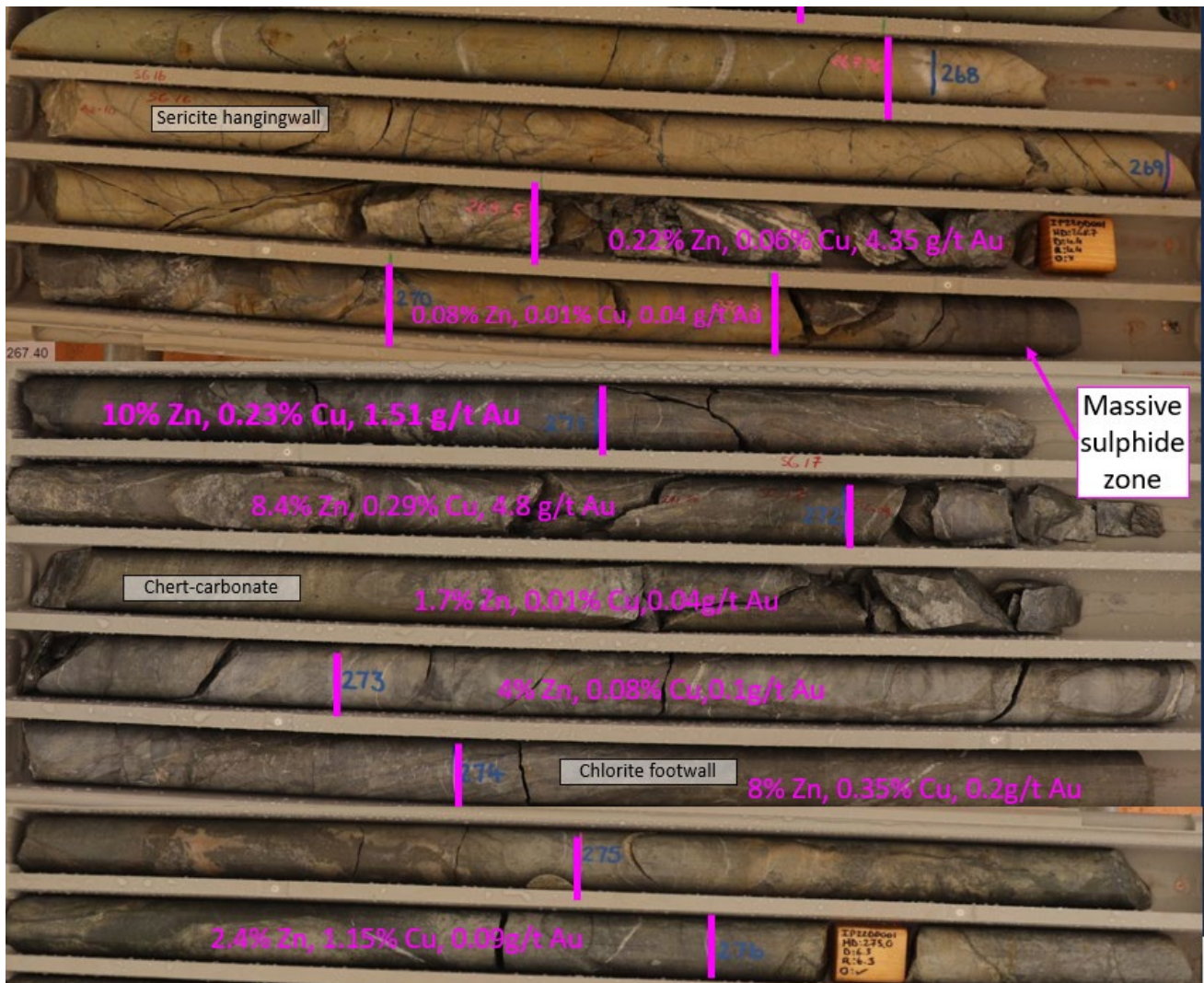
Figure 3: IP22DD001 core showing sample intervals and latest results along with previous gold results (reported in ASX announcement 15 December 2022).
